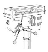
FIGURE 11. INSTALLING THE FEED HANDLES
